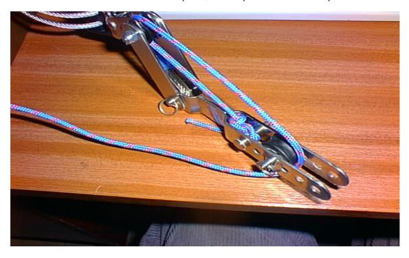
Adjust the cord tension so that all slack is removed in the fast trim position. It may then be necessary to adjust the trim indicator position to give correct trim speed indication.
